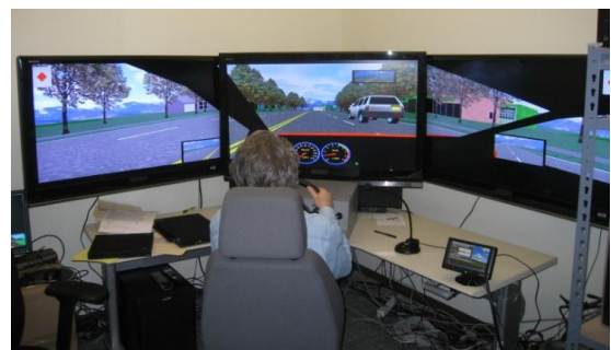
Figure 1: The STISim driving simulator. The system hosts a console with a steering wheel, turn signals, and buttons mapped to external functions. Three 47" screens placed at roughly 45° generate a convincing impression of driving a vehicle.
